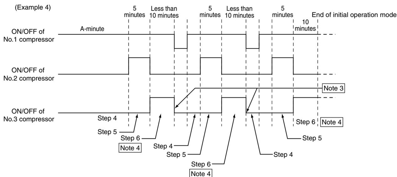
Note 1: If Step 4 is interrupted (compressor stopped by thermostat OFF or regular stop), Step 4 will be redone at restart.
