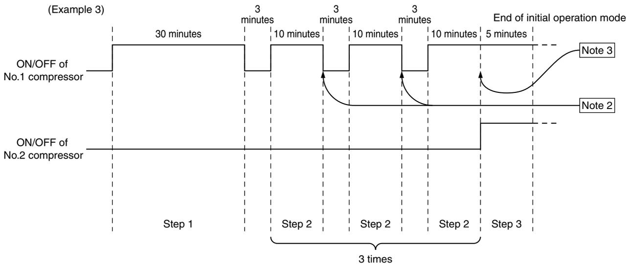
Note 1: If the frequency of No. 1 compressor is above the specified level at the end of Step 2, the mode proceeds to Step 3.
