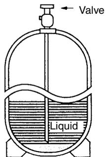
For a cylinder without a syphon attached
