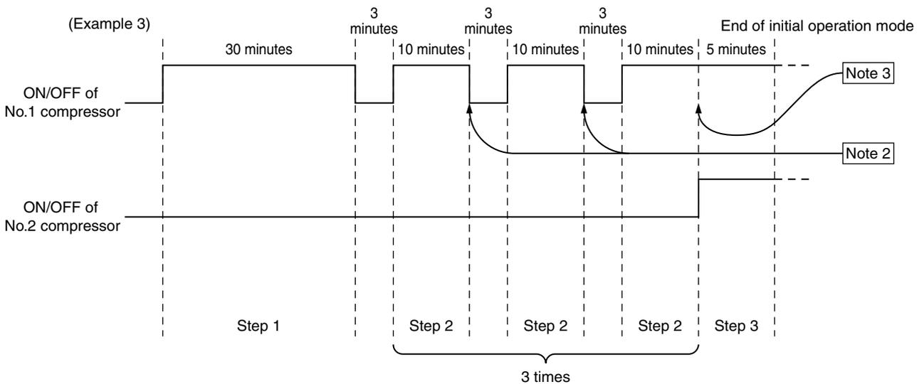
Note 1: If the frequency of No. 1 compressor is above the specified level at the end of Step 2, the mode proceeds to Step 3.
