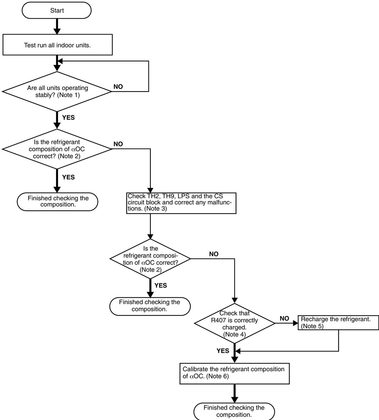
Note 1 Wait until the units stabilize as described in the refrigerant amount adjustment procedure in “Chapter 6”.
