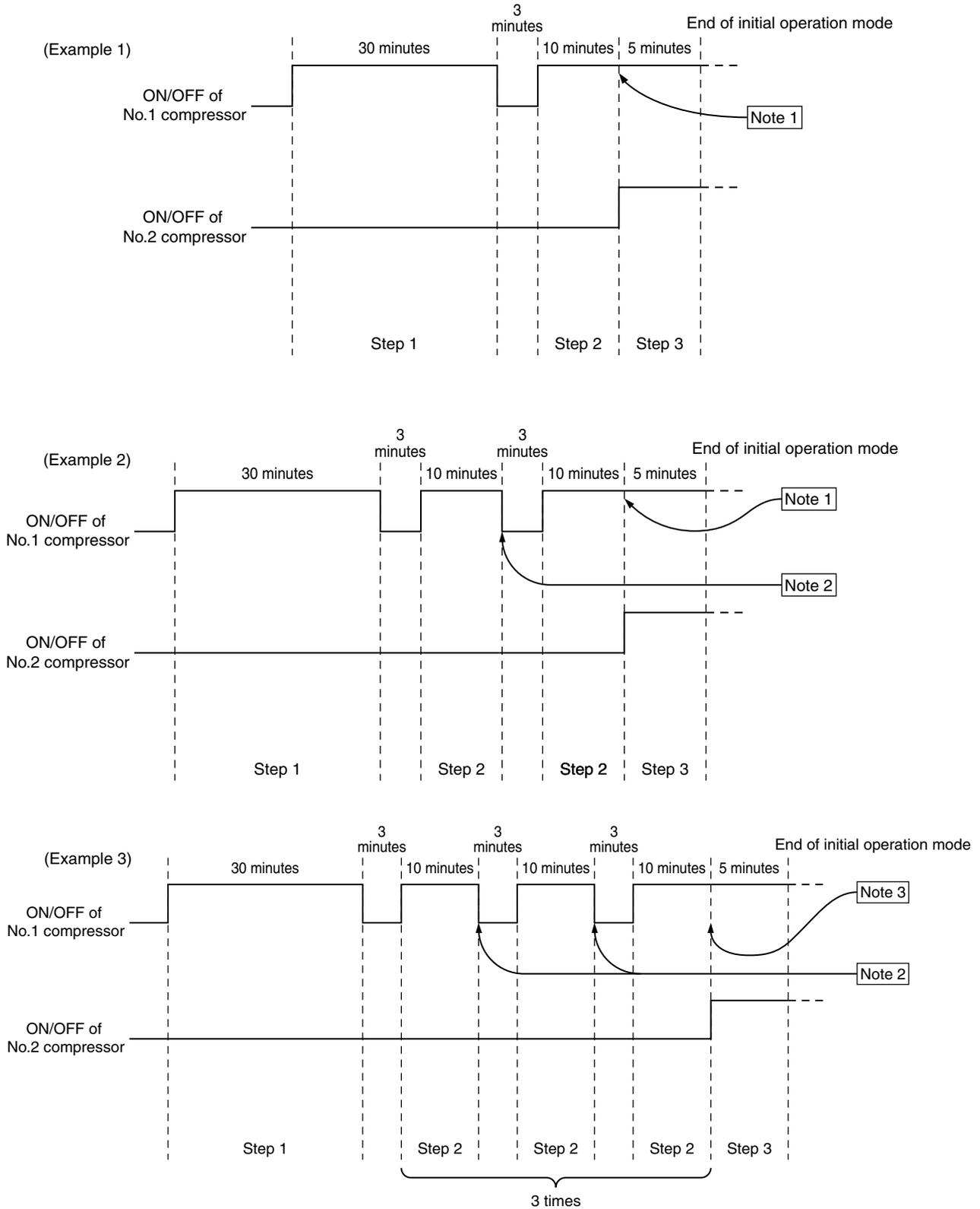
Note 1: If the frequency of No. 1 compressor is above the specified level at the end of Step 2, the mode proceeds to Step 3.
