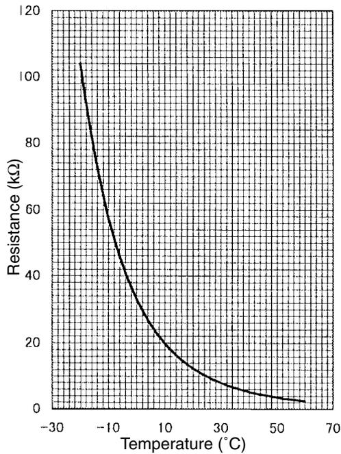
Thermistor  $R_{50} = 17\text{k}\Omega \pm 2\%$  (THHS)
