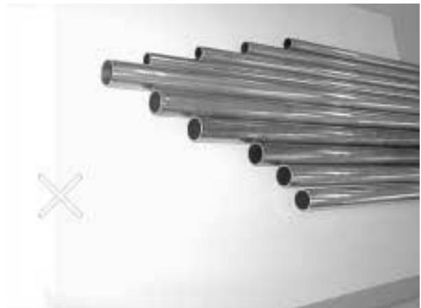
Both ends of the pipes should be sealed until immediately before brazing.
