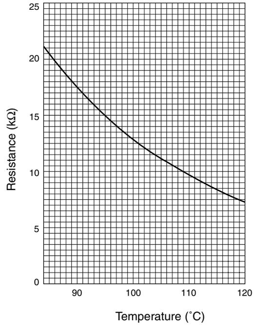
Thermistor  $R_0 = 33\text{k}\Omega \pm 1\%$  (TH2)
