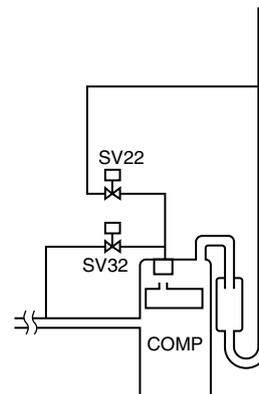
**(5) Oil return control (Electronic expansion valve (SLEV))**
