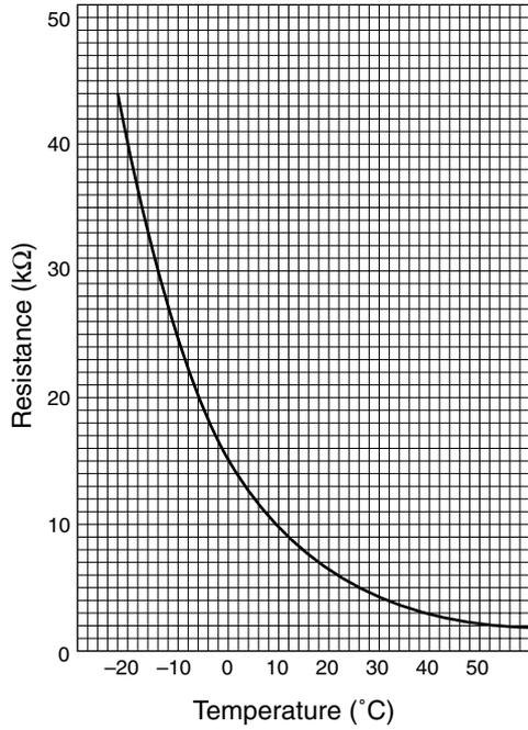
Thermistor  $R_{120} = 7.465\text{k}\Omega \pm 2\%$  (TH11,12,10c)
