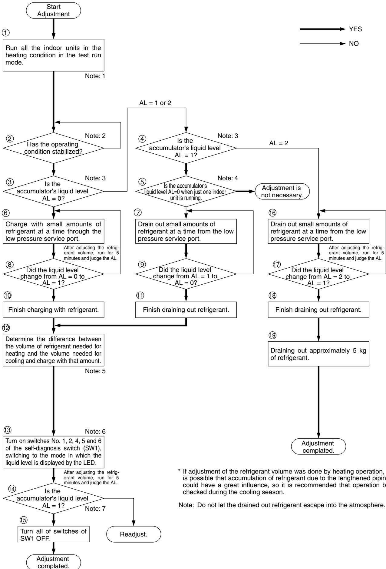
\* If adjustment of the refrigerant volume was done by heating operation, it is possible that accumulation of refrigerant due to the lengthened piping could have a great influence, so it is recommended that operation be checked during the cooling season.
