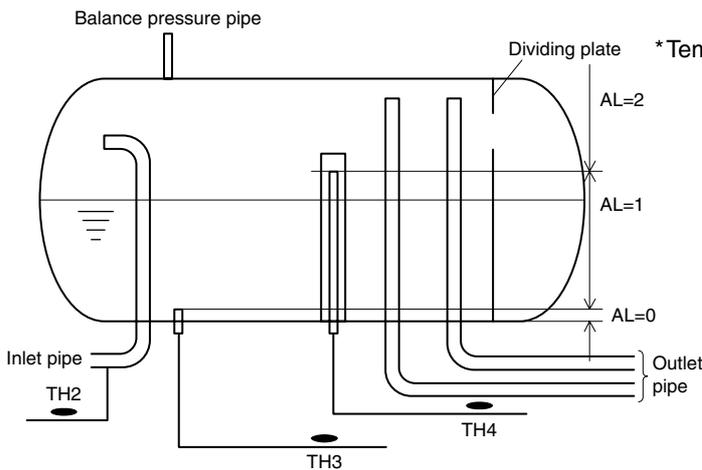
\* Temperature A: low pressure saturation temperature.
